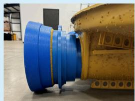
Precaster's casting the baseliner upside down ensures 4000+ PSI throughout entire structure, including benching, in one step; increasing production speed by eliminating benching by hand later.
